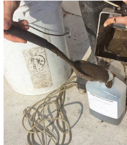
Sediment samples were transferred into a Nalgene bottle in order to transport sediment samples to Aquatic Systems, where larval counting took place
